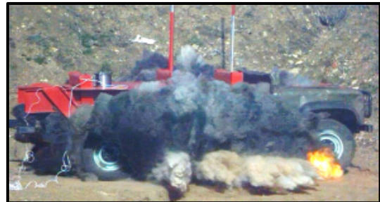
Figure. 12: Time 5ms – Gas ejecta cloud 4m diameter
