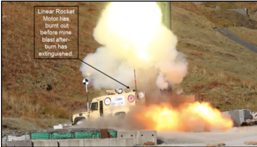
Figure. 30: AMPS™ – Active Mine Protection System Proof of Concept Test.
