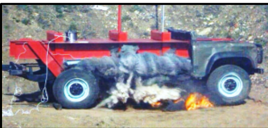
Figure. 10: Time 3ms – Gas ejecta cloud 2m diameter.
