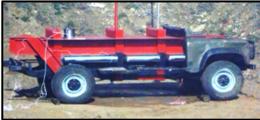
Figure. 7: UK MOD funded baseline vehicle VGAM test. Time zero – detonator igniting.
