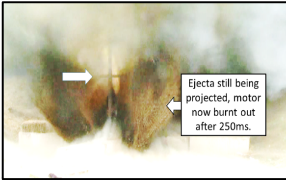
Figure. 14: Duration of Mine Blast Ejecta Projection.
