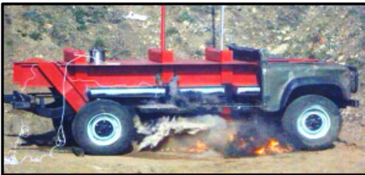
Figure. 9: Time 2ms – Gas ejecta cloud 1m diameter
