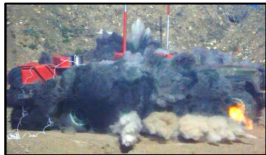
Figure. 13: Time 6ms – Gas ejecta cloud 5m diameter
