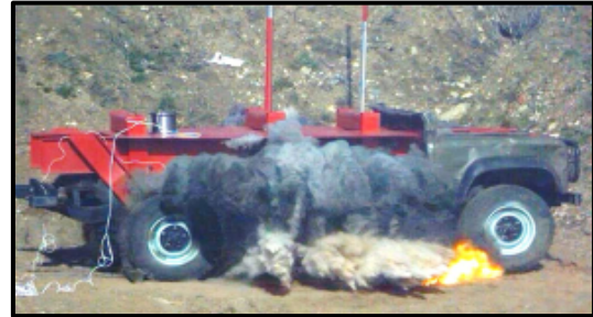
Figure. 11: Time 4ms – Gas ejecta cloud 3m diameter
